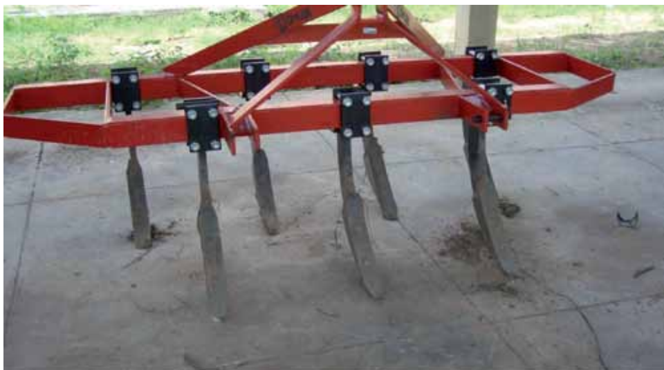
Photo 32- Scarifier for surface decompaction
