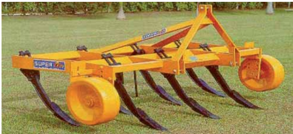
Photo 33 - Deep Soil Plough for Deep Decompaction
